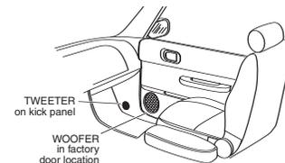
**Figure 3.** Mounting the woofer in the door and the tweeter in the A-pillar.
