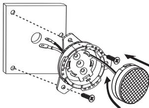
**Figure 7B.** Flush-mounted to surface behind grille panel.
