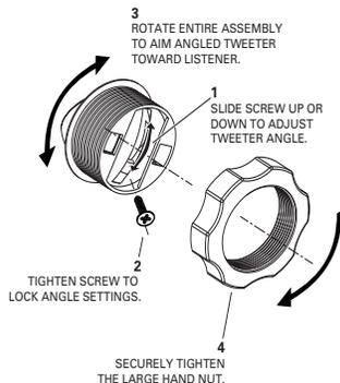
**Figures 7A through 7D.** The Starfish™ tweeter mount is intended to be used when the tweeter will be installed behind a factory grille (e.g., replacing the factory tweeter behind a door panel). The Starfish will allow you to mount the component tweeter directly to the panel itself or to the area behind the panel. The six mounting tabs can be removed easily to create a number of custom configurations.
